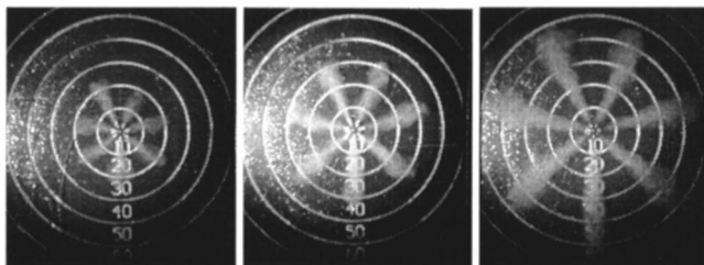
Fig. 32 Maximum penetration length of pilot injection with various injection pressure; 25 MPa (left), 30 MPa (middle), and 50 MPa (right)
