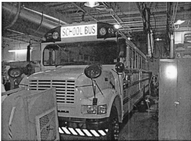
Fig. 1 1996 Carpenter school bus installed on SwRI heavy-duty chassis dynamometer
